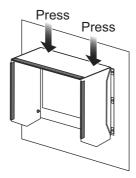
9. Set the hood (19) assembly with the knobs tightly (4 pcs.).
